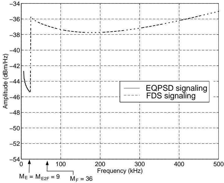
Figure 18: *Optimal upstream transmit spectrum for CSA Loop 6 (HDSL2 transmit spectrum with 39 self-NEXT + 39 self-FEXT). EQPSD signaling takes place to the left of bin 9 (indicated by solid line); FDS signaling takes place to the right (indicated by dashed line).*
