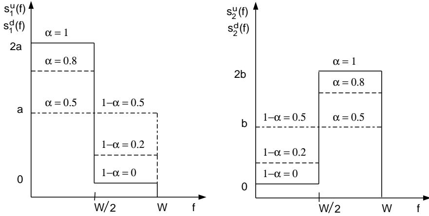
Figure 31: *Different line characteristics: Upstream and downstream transmit spectra in a single frequency bin ( $\alpha = 0.5 \Rightarrow$  EQPSD signaling and  $\alpha = 1 \Rightarrow$  multi-line FDS signaling).*
