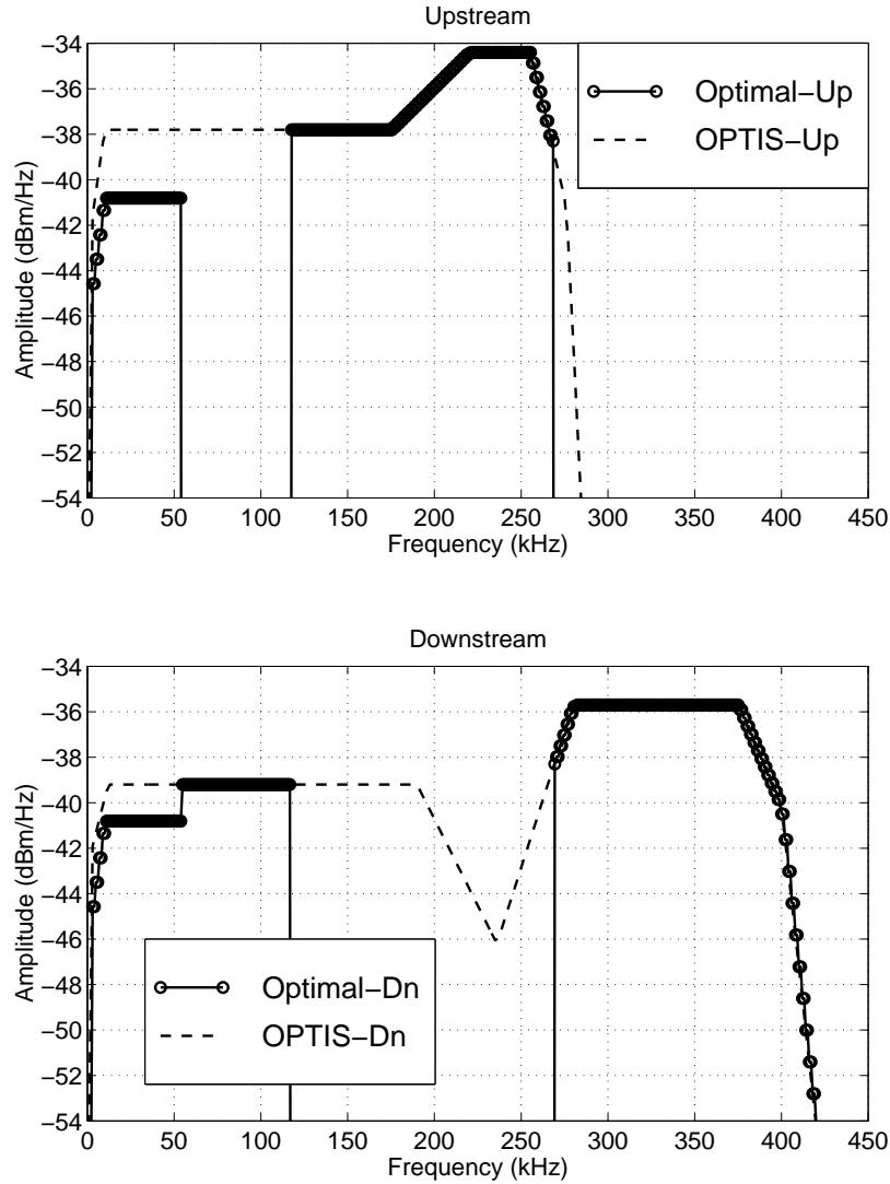
Figure 35: Optimal upstream and downstream transmit spectra for HDSL2 (on CSA loop 6) under the OPTIS upstream and downstream constraining PSD masks with 24 HDSL2 self-NEXT and self-FEXT interferers, 24 T1 interferers, and AGN of  $-140$  dBm/Hz. The ‘o—o’ lines show the peak-constrained optimal transmit spectra and the ‘---’ lines show the constraining OPTIS PSD masks.
