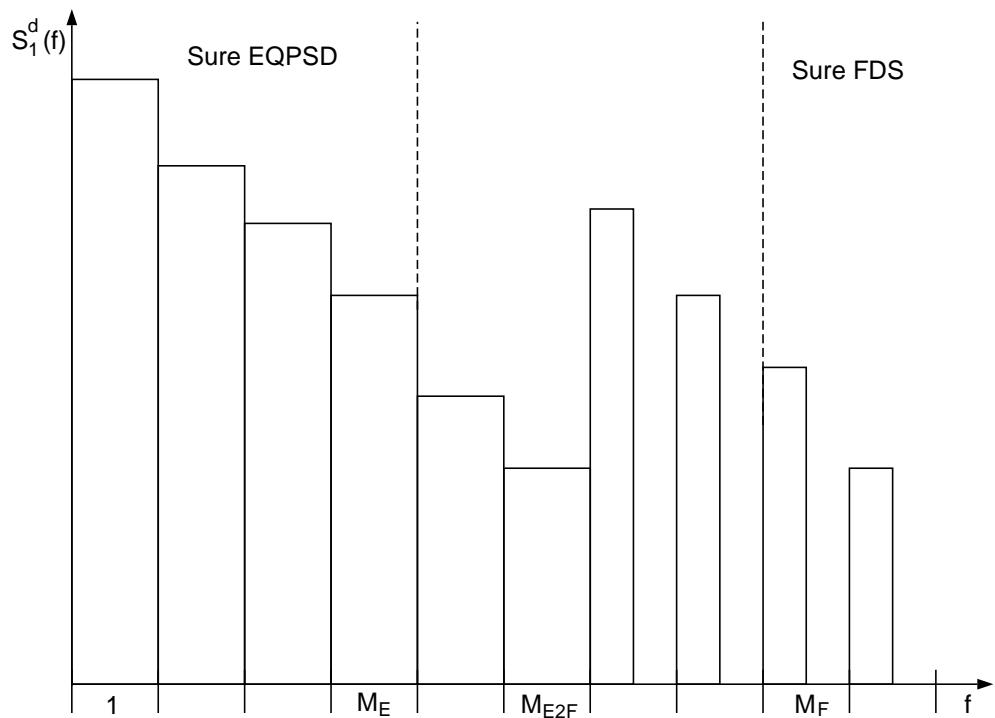
Figure 15: Upstream and downstream transmit spectra showing regions employing EQPSD and FDS signaling. The bins  $[1, M_{E2F}]$  employ EQPSD signaling and the bins  $[M_{E2F} + 1, K]$  employ FDS signaling.
