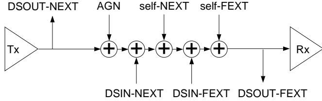
Figure 3: *NEXT* (*DSIN-NEXT* and *self-NEXT*), and *FEXT* (*DSIN-FEXT* and *self-FEXT*) modeled as additive interference sources. *AGN* denotes the additive Gaussian channel noise. *DSOUT-NEXT* and *DSOUT-FEXT* represent the interference leaking out into other neighboring services.
