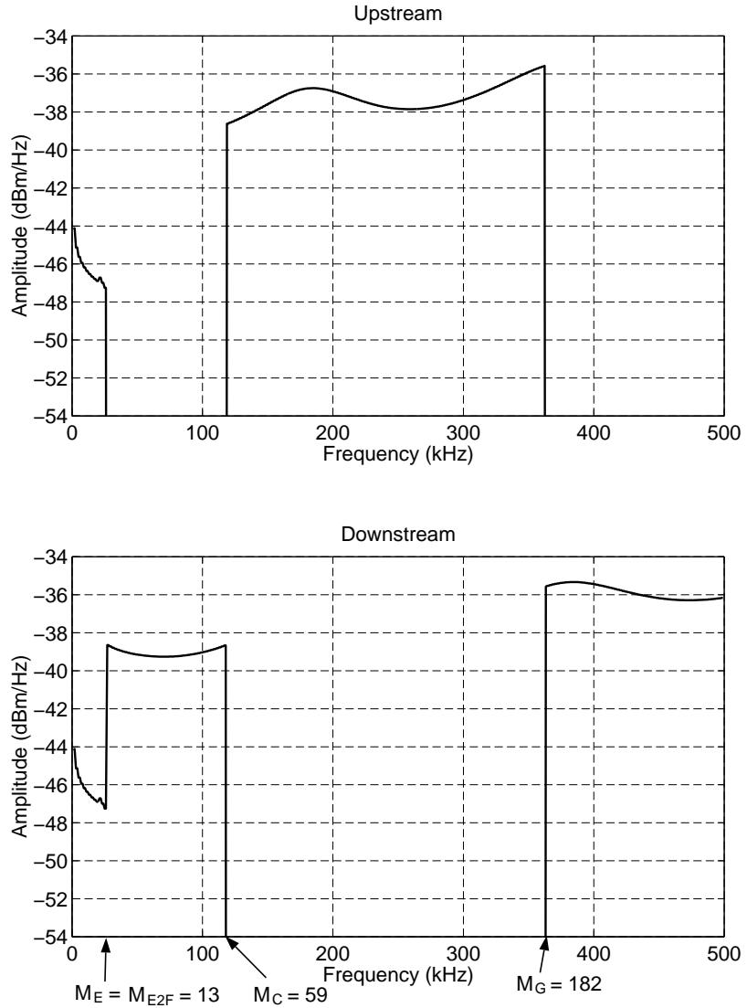
Figure 36: Optimal “contiguous” upstream and downstream transmit spectra for CSA Loop 4 (having a non-monotonic channel transfer function due to bridged taps ) (HDSL2 transmit spectrum with 39 self-NEXT + 39 self-FEXT). These spectra yield equal performance margins (equal capacities) and equal average powers in both directions of transmission. Note that there is only one transition region from EQPSD to FDS signaling.
