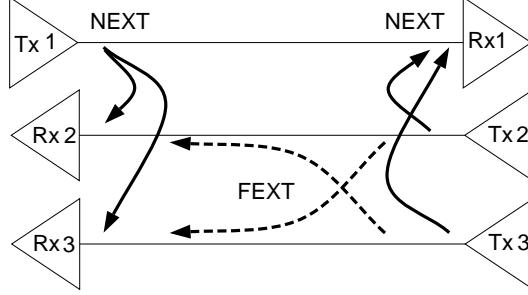
Figure 2: *NEXT* and *FEXT* between neighboring lines in a telephone cable. *Tx*'s are transmitters and *Rx*'s are receivers.
