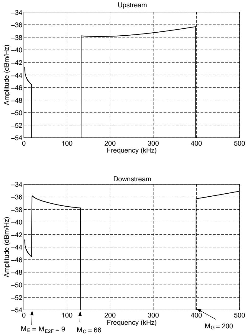
Figure 20: Another set of optimal “contiguous” upstream and downstream transmit spectra for CSA Loop 6 (HDSL2 transmit spectrum with 39 self-NEXT + 39 self-FEXT). These spectra yield equal performance margins (equal capacities) and equal average powers in both directions of transmission. EQPSD signaling takes place to the left of bin 9.
