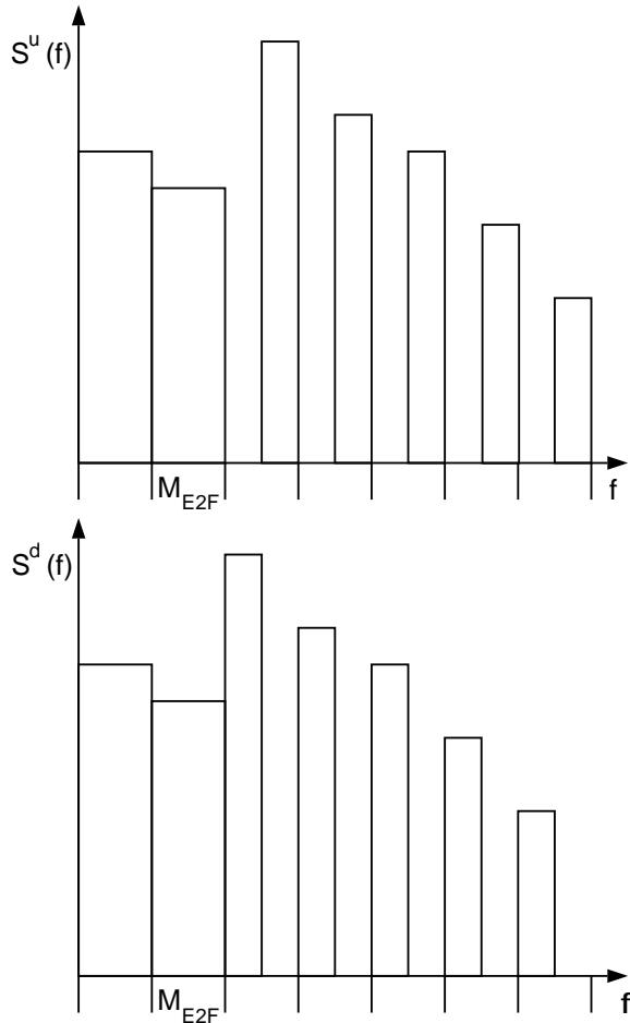
EQPSD/FDS with "discrete" transmit spectra
