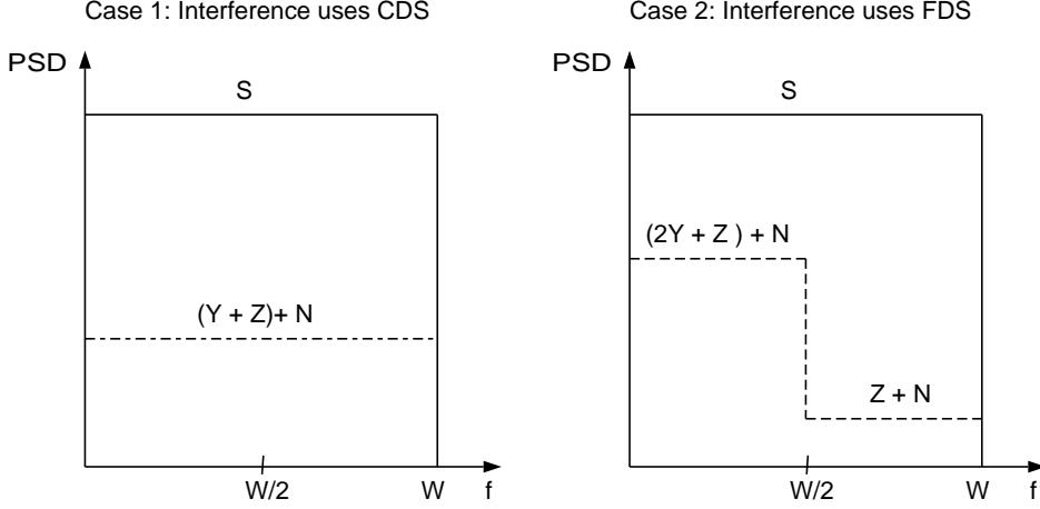
Figure 21: *Transmit spectra of signaling line ( $S$ ), interfering line ( $Y$  and  $Z$ ), and lumped channel noise ( $N$ ). FDS scheme (Case 2) for interfering line yields higher capacity for signaling line ( $S$ ) than other schemes like CDS (Case 1).*
