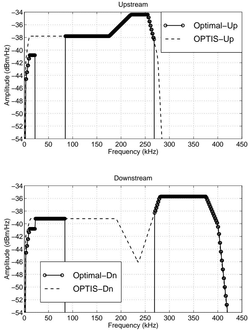
Figure 34: Optimal upstream and downstream transmit spectra for HDSL2 (on CSA loop 6) under the OPTIS upstream and downstream constraining PSD masks with 39 HDSL2 self-NEXT and self-FEXT interferers and AGN of  $-140$  dBm/Hz. The ‘o—o’ lines show the peak-constrained optimal transmit spectra and the ‘---’ lines show the constraining OPTIS PSD masks.
