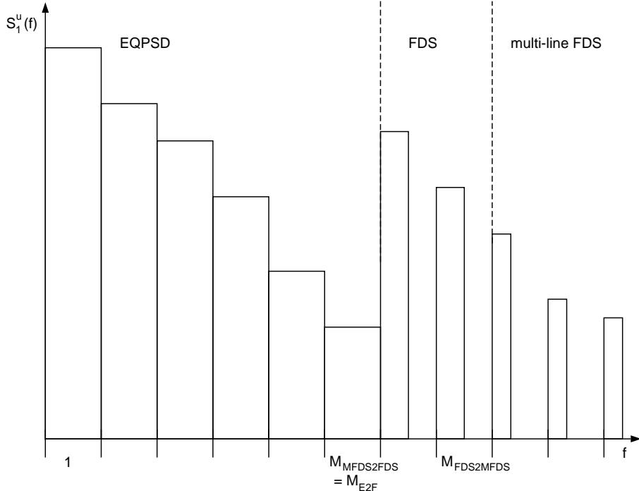
Figure 26: Practical observation number 2: Bins  $[1, M_{MFDS2FDS}]$  employ EQPSD, bins  $[M_{MFDS2FDS} + 1, M_{FDS2MFDS}]$  employ FDS, and bins  $[M_{FDS2MFDS} + 1, K]$  employ multi-line FDS. There is no multi-line FDS spectral portion within the EQPSD region.
