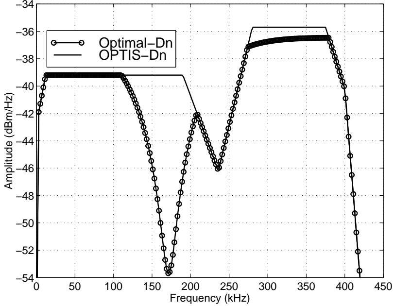
Figure 32: Optimal downstream transmit spectrum of HDSL2 (on CSA loop 6) under an OPTIS downstream constraining PSD mask with 49 HDSL DSIN-NEXT interferers and AGN of  $-140$  dBm/Hz. The ‘o—o’ line shows the peak-constrained optimal transmit spectrum and the ‘—’ line shows the constraining OPTIS PSD mask.
