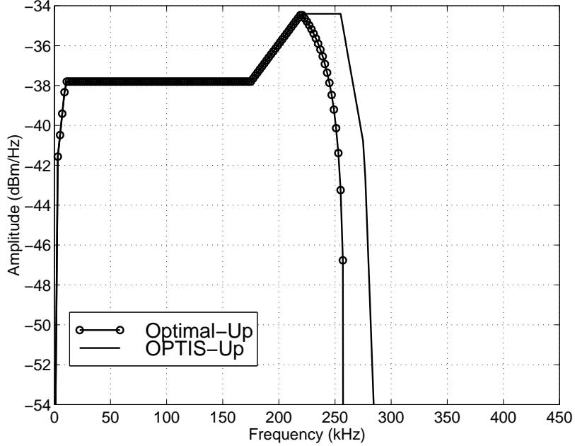
Figure 33: Optimal upstream transmit spectrum for HDSL2 (on CSA loop 6) under an OPTIS upstream constraining PSD mask with 25 T1 DSIN-NEXT interferers and AGN of  $-140$  dBm/Hz. The ‘o—o’ line shows the peak-constrained optimal transmit spectrum and the ‘—’ line shows the constraining OPTIS PSD mask.
