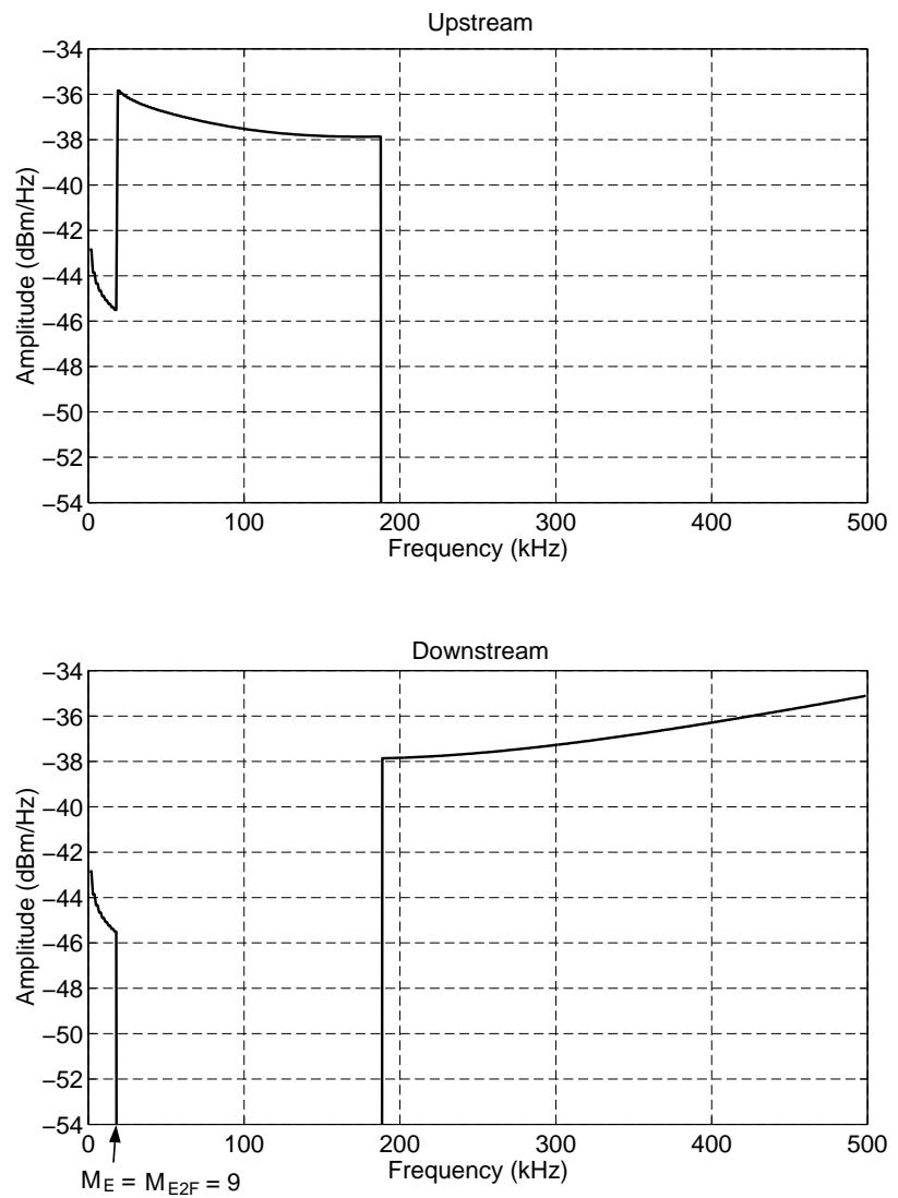
Figure 19: Optimal “contiguous” upstream and downstream transmit spectra for CSA Loop 6 (HDSL2 transmit spectrum with 39 self-NEXT + 39 self-FEXT). EQPSD signaling takes place to the left of bin 9.
