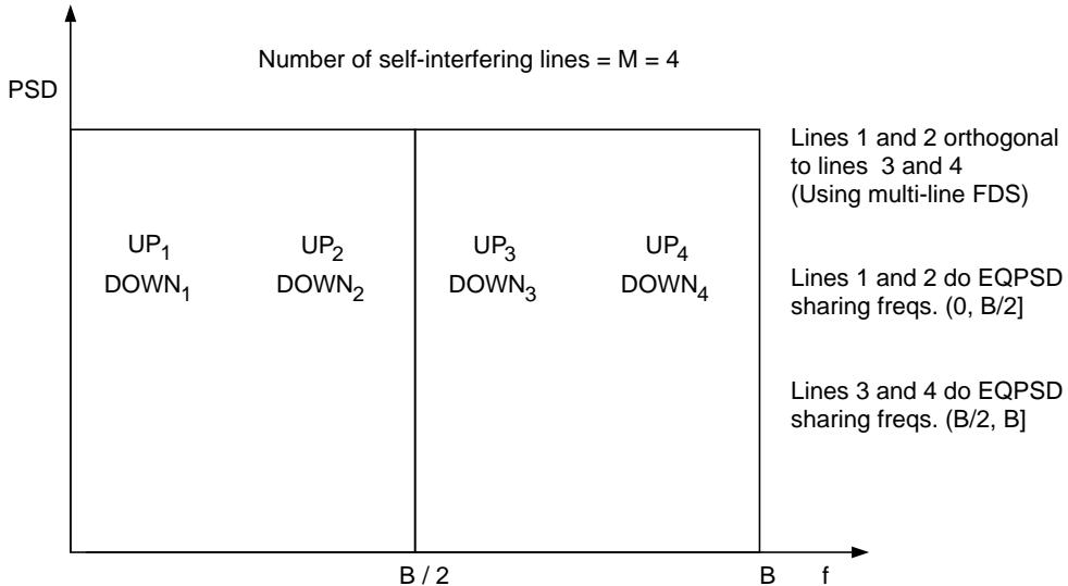
Figure 38: *Alternative signaling scheme: In presence of high degrees of self-NEXT and self-FEXT between group of lines 1 and 2 and lines 3 and 4 we employ multi-line FDS. There is EQPSD signaling within each group of lines (1 and 2 employ EQPSD as do 3 and 4) that have low self-interference.*
