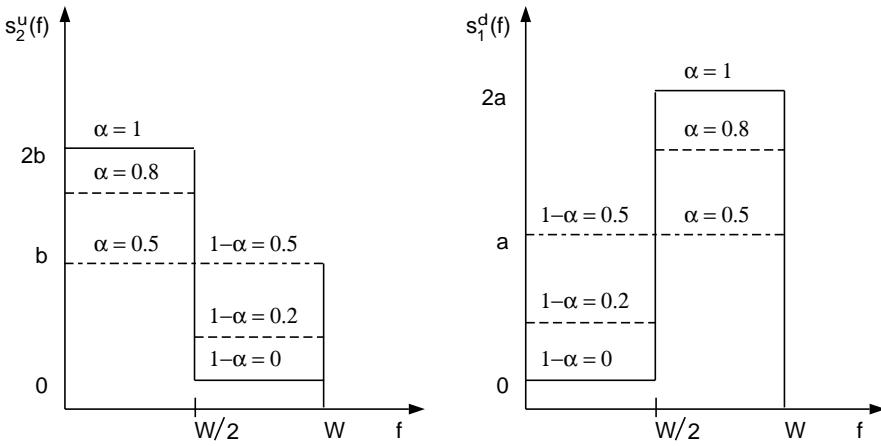
Figure 30: Different line characteristics: Upstream and downstream transmit spectra in a single frequency bin ( $\alpha = 0.5 \Rightarrow$  EQPSD signaling and  $\alpha = 1 \Rightarrow$  FDS signaling).
