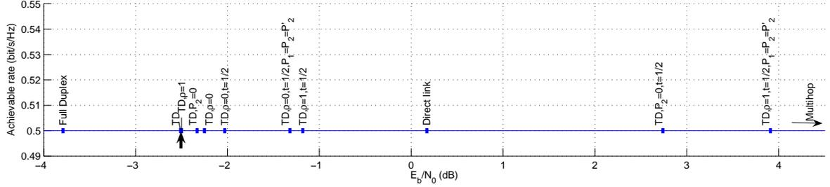
Fig. 2. Minimal  $E_b/N_0$  in dB required for an error-free transmission with binary rate-1/2 coded inputs with several constraints. The arrow indicates the near-optimal scheme that we select in this paper: optimal time-sharing and power allocation and fully correlated source and relay signals in the second phase ( $\rho = 1$ ).
