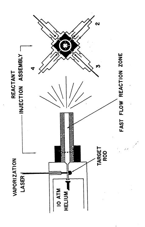
the 400  $\mu s$  of the main nozzle pulse. The annular reservoir served as a gas ballast feeding each of the four injection needles equally, thus ensuring that the flow of reactant into the reaction tube is independent of which nozzle is fired.
