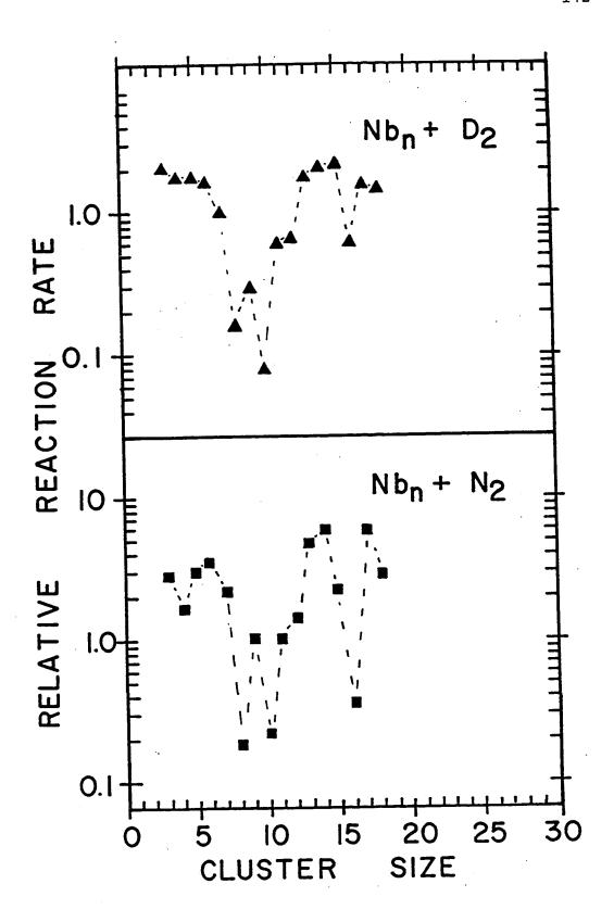
3-9 size range. Note, for example, that the niobium trimer has nearly disappeared from the mass spectrum, the missing ion signal reappearing in peaks corresponding to  $\mathrm{Nb_3N_2}$ ,  $\mathrm{Nb_3N_4}$ , and  $\mathrm{Nb_3N_6}$ . In sharp contrast, the  $\mathrm{Nb_8}$  cluster has been largely unaffected by the  $\mathrm{N_2}$  reactant.
