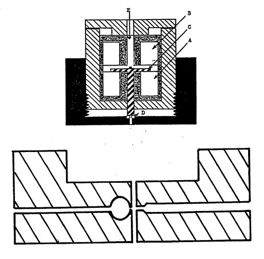
extends through a bronze bearing fit within the center of the front (close) coil. The face of the plunger is what actually seals against an o-ring (Parker 0.002-2) on the face plate of the nozzle housing.
