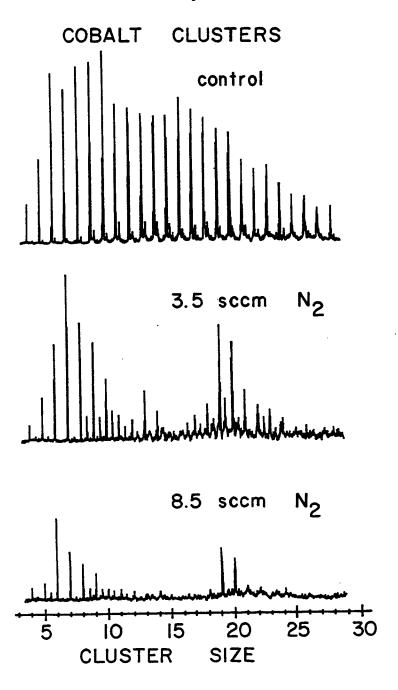
Figure 26. Relative reaction rates of cobalt clusters with  $D_2$  and  $N_2$ . Note the striking similarity in the reactivity patterns for these two reactants. The estimated errors for these relative rates is  $\pm 20\%$  except for rates greater than 10 or less than 0.1 compared to the reference rate; for these extreme rates the measurements are only of semi-quantitative significance.
