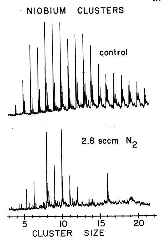
Figure 29. Detail of small cluster region of the  $\mathrm{N}_2$  chemisorption study on niobium. Peaks due to  $\mathrm{N}_2$  chemisorption reaction products have been blackened in for emphasis. Note that the reactivity of the  $\mathrm{Nb}_n\mathrm{O}$  oxides is often markedly different from the corresponding pure niobium clusters -- see the  $\mathrm{Nb}_3$  and  $\mathrm{Nb}_8$  clusters particularly in this regard.
