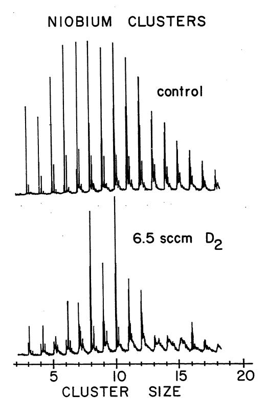
Figure 28. Chemisorption study of  $N_2$  on niobium clusters. The sharp peaks in the small cluster region of the lower mass spectrum are due to the  $N_2$  chemisorption product, whereas the peaks seen in roughly the correct position for the 8-12 and 16th cluster of niobium are, in fact, due to the unreacted cluster.
