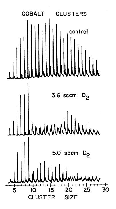
very dramatic size dependencies in their reaction with  $D_2$ . Note particularly the rapid onset of high reactivity on going from 9 to 10 atoms per cluster. At the time it was first discovered, this was the most abrupt change ever observed in <u>any</u> property of a metal cluster as a function of size.
