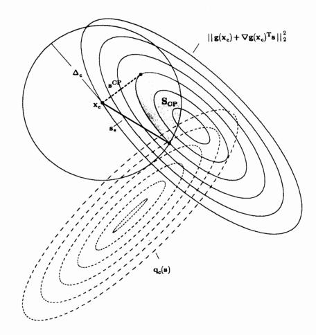
FIGURE 4.1 A Constrained Trust Region Step
