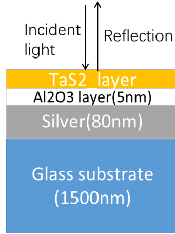
Figure 4.6 : Optical Limiter structure in detail.
