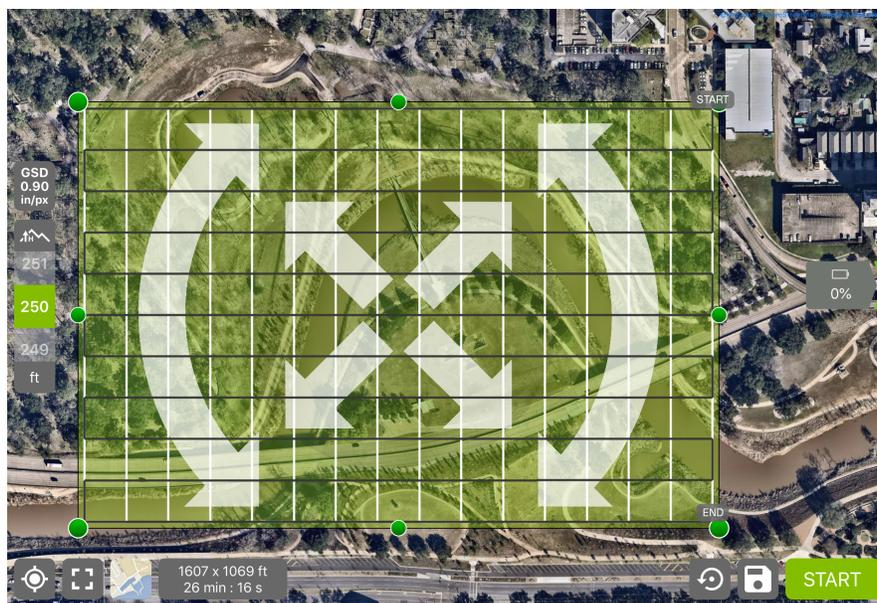
**Figure 2.** Screenshot from original 2/16/19 flight plan for Buffalo Bayou study site. Figure shows double grid feature, Ground Sampling Distance (GSD), adjustable flight elevation, area of flight, and estimated flight time.
