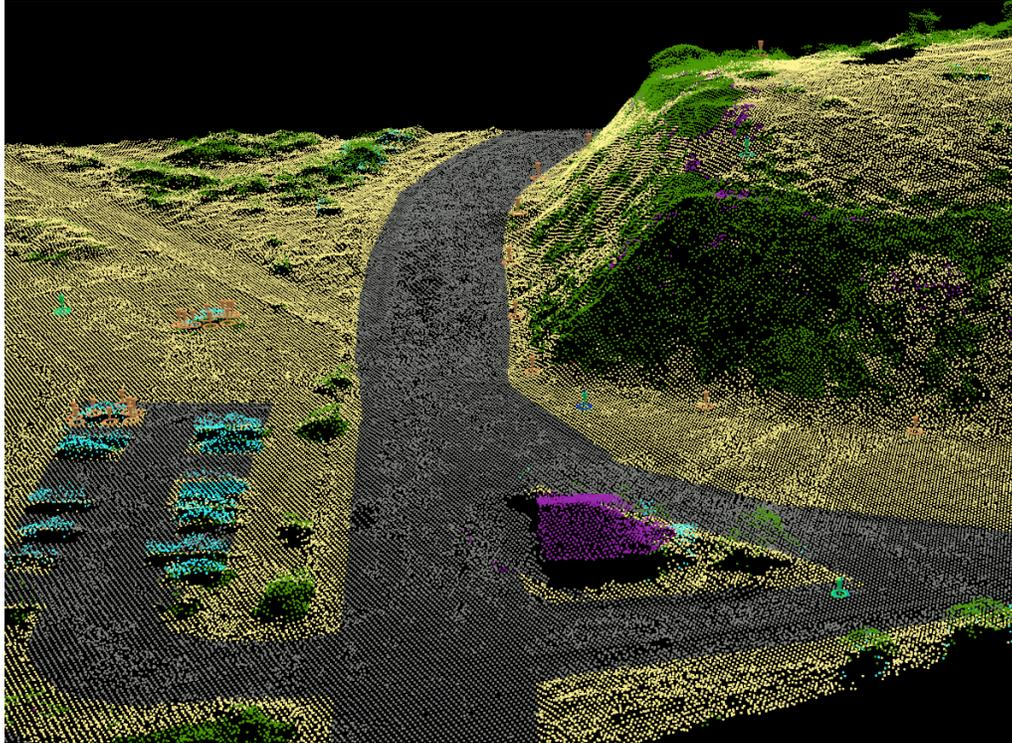
**Figure 7.** Complete classification of a point cloud. Initial classification was generated by Pix4D and then edited by Jessica Sheldon. Yellow represents ground, green is high vegetation, gray is road surface, purple is man-made object, and blue is unclassified which in this model indicates vehicle.
