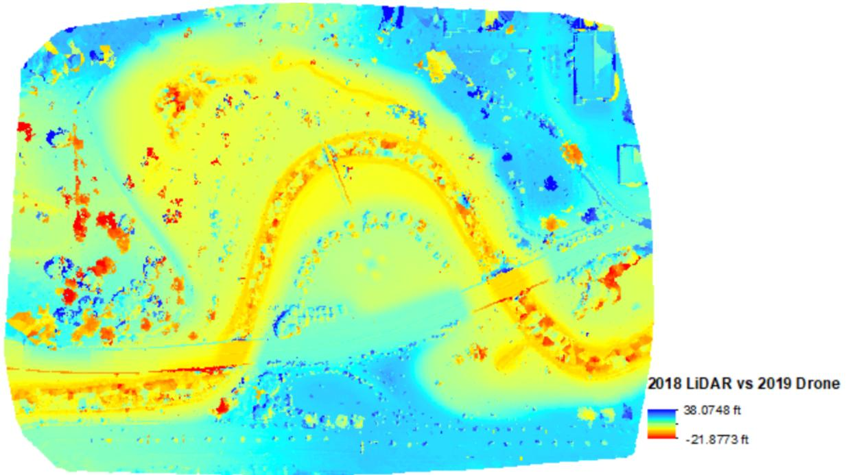
**Figure 6B.** GIS created difference map. 2018 LiDAR DEM vs 2019 calibrated DEM.
