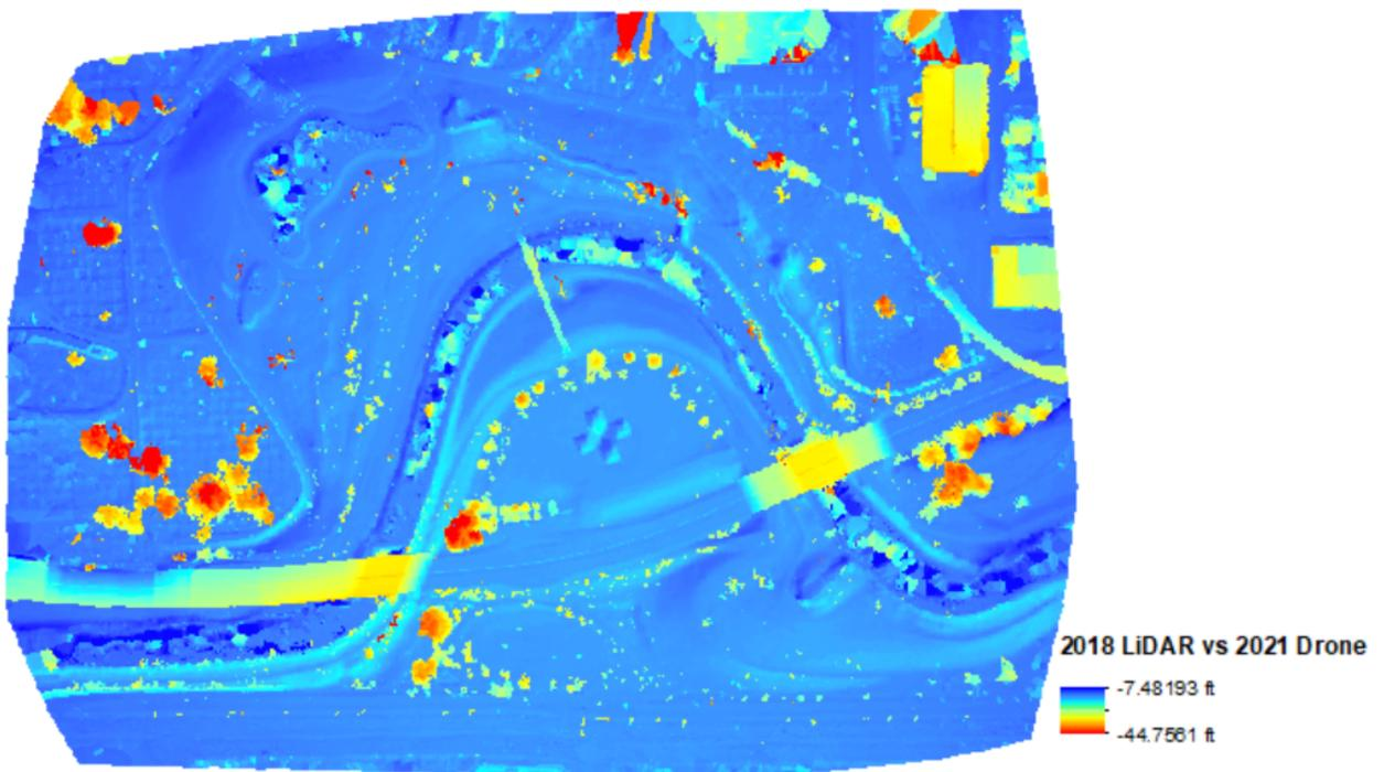
**Figure 6C.** GIS created difference map. 2018 LiDAR DEM vs 2021 calibrated DEM.
