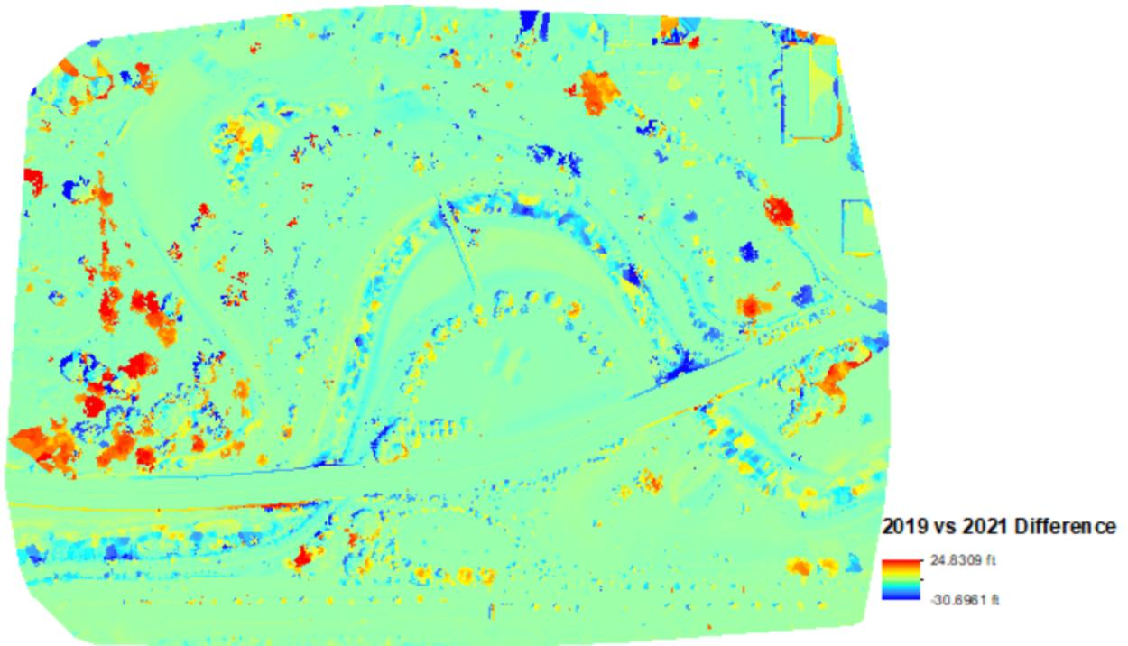
**Figure 6A.** GIS created difference map. 2019 calibrated DEM vs 2021 calibrated DEM.
