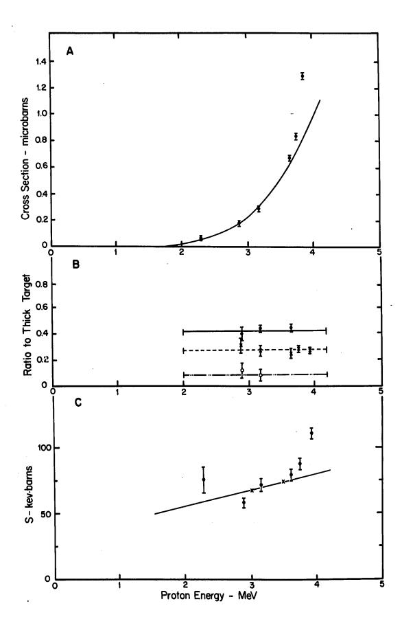
The values of the cross-section obtained by TT are indicated in Figure 12 and are in good agreement with the measured value. The cross-section, calculated assuming the energy dependence given by CD, but normalized to the results of TT, is shown and reproduces the general trend of the data. The energy dependence of S obtained by CD was used for this calculation and for Ca<sup>40</sup> is of the form:
