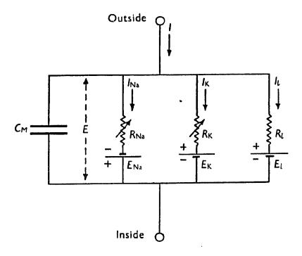
$$\begin{split} I = C_M \frac{\mathrm{d}\,V}{\mathrm{d}t} + \bar{g}_\mathrm{K} n^4 \, (V - V_\mathrm{K}) + \bar{g}_\mathrm{Na} m^3 h \, (V - V_\mathrm{Nu}) + \bar{g}_l \, (V - V_l), \\ \mathrm{d}n/\mathrm{d}t = \alpha_n (1 - n) - \beta_n n, \\ \mathrm{d}m/\mathrm{d}t = \alpha_m (1 - m) - \beta_m m, \\ \mathrm{d}h/\mathrm{d}t = \alpha_h (1 - h) - \beta_h h, \end{split}$$
