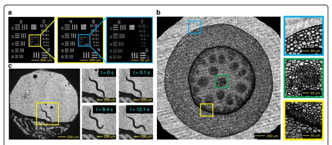
**Fig. 5 WISH for lensless microscopic imaging. a** Reconstruction of a USAF resolution target with a large FOV (5 mm × 5 mm) and a high resolution (4.92 μm bar width). **b** The reconstruction of a cross-section of the lily-of-the-valley. Three zoomed-in images show details of the characteristic regions. **c** Four frames from a reconstructed video (10 Hz) of a Caenorhabditis elegans living on agar
