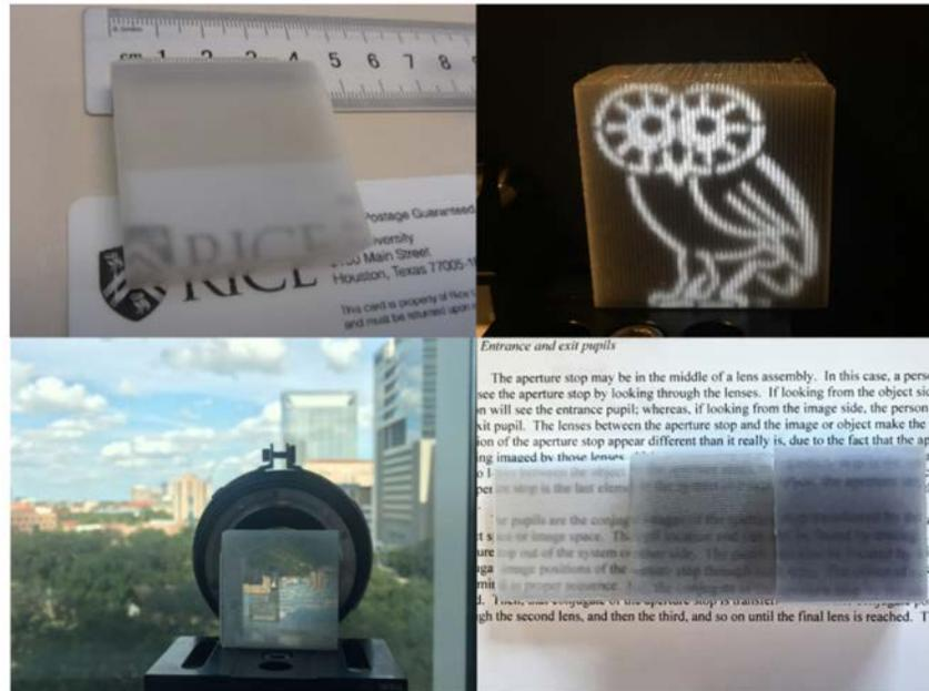
Fig. 12. The image guiding capability of 3D printed faceplates for various macro features: (a) A Rice student identification card. (b) A laser-cut image mask of a Rice mascot owl logo at the input surface which is illuminated by a white-light LED. (c) A university campus view captured at the image plane of a photographic objective (Sigma 85mm f/1.4 EX DG HSM). (d) Image guiding capability comparison for various fiber lengths (from left to right: 10mm, 30mm, and 50mm)
