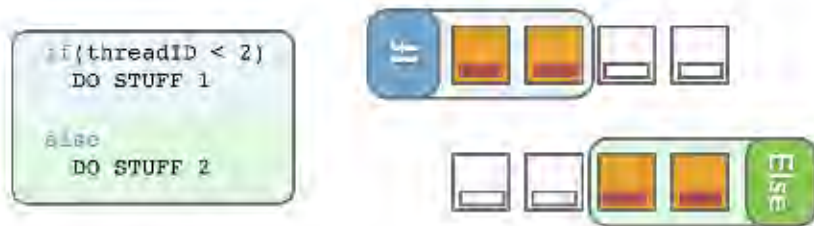
Figure 2.5: Work-items on the same hardware groups (half-warp or wavefront) follow the same instruction or call a NOOP (No Operation) instruction.
