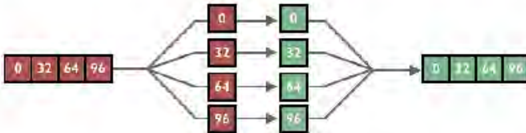
Figure 2.3: With large registers and vectorization instructions, multiple consecutive data entries can be updated in parallel.
