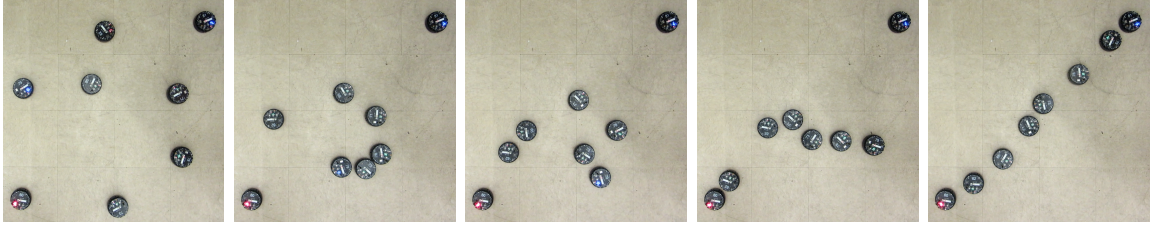
Figure 5.8 : Physical sorting with eight robots. Collision and interference happened, but robots managed to get sorted.
